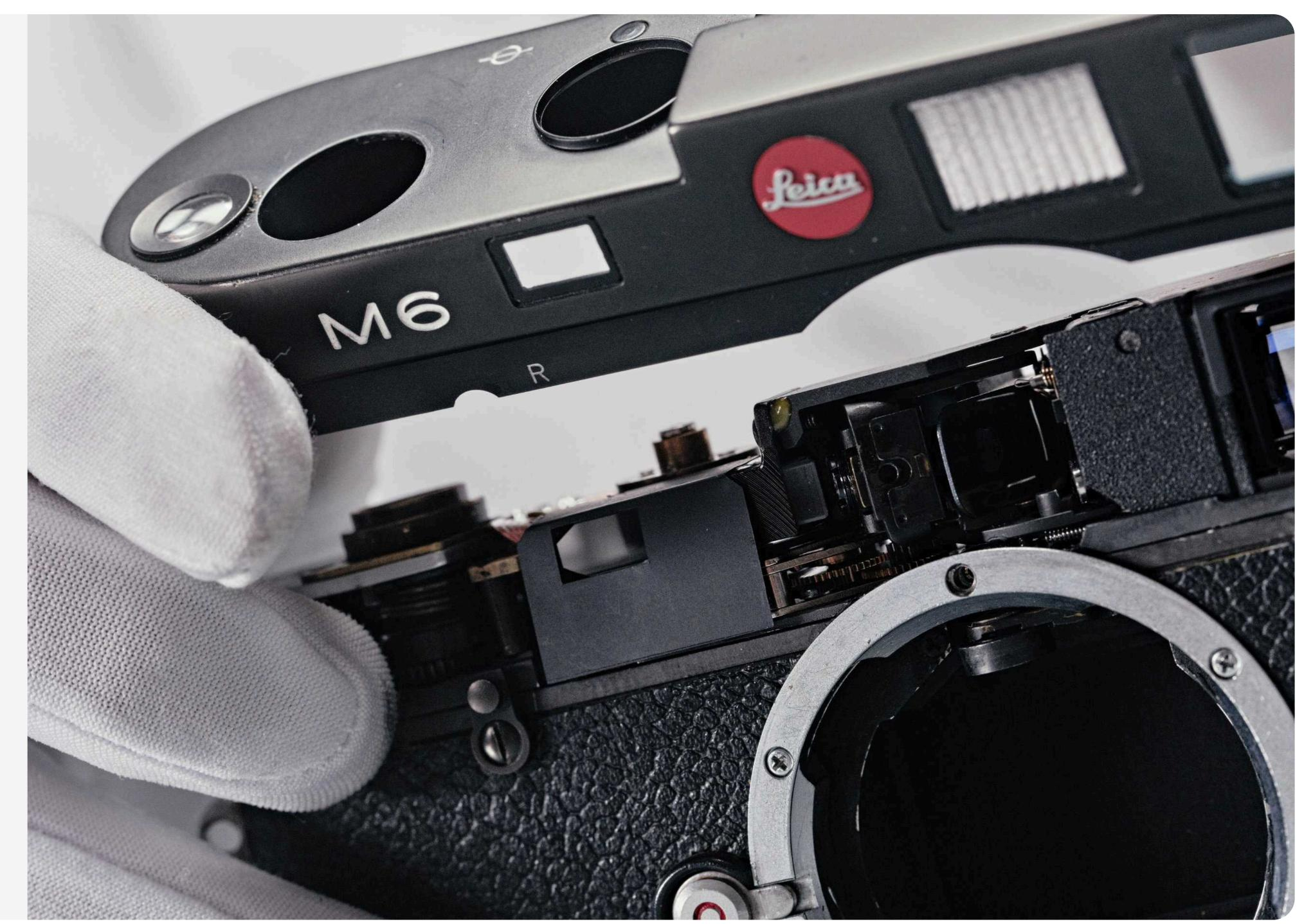
We disassemble the light meter unit, inspect all components, and clean electrical contacts to ensure proper conductivity. Faulty parts, such as the photocell or resistor, are repaired or replaced with high-quality components. The meter is then recalibrated using precision light sources to guarantee accurate readings across the entire EV range. We adjust the system to match the original Leica specifications, ensuring reliable performance with modern batteries.
